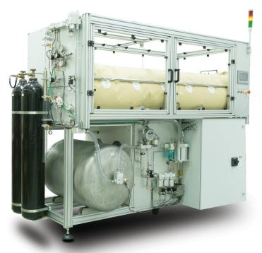
The recovery system collects helium from the test part, where it is first pumped into a low-pressure holding tank. The helium then flows through a compressor and is stored in a high-pressure supply tank, which enables the charging station to reuse helium in the subsequent part's testing. Dependent on the performed test type, it is possible to recover and reuse up to 98% of the helium.
